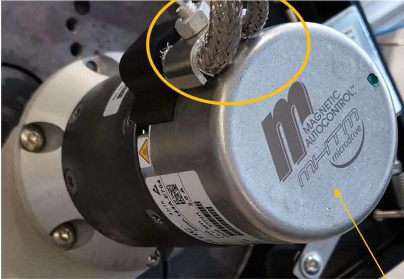
The MHP1 cable exit is pointed away from the motor shaft.
