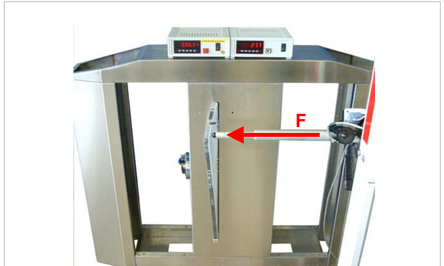
Fig. 3-1 Static test, figure shows a deformation of 27 mm at static force of 500 N
