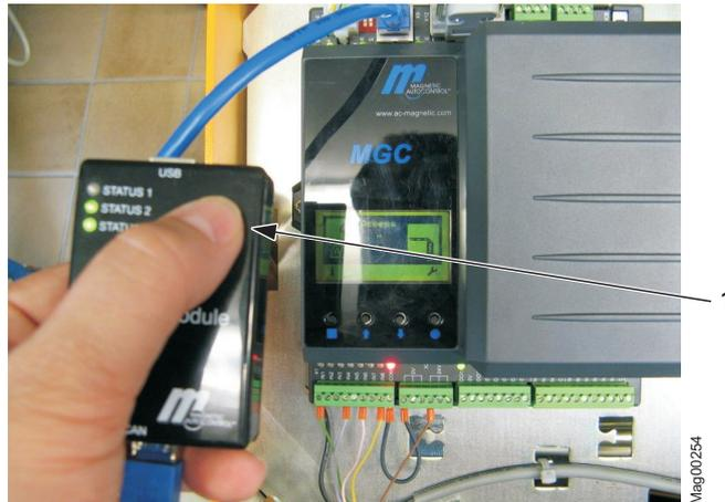
Fig. 4: Press the push button at the service module
