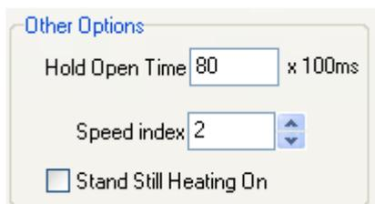
Fig. 8.9: Setting the hold-open time
