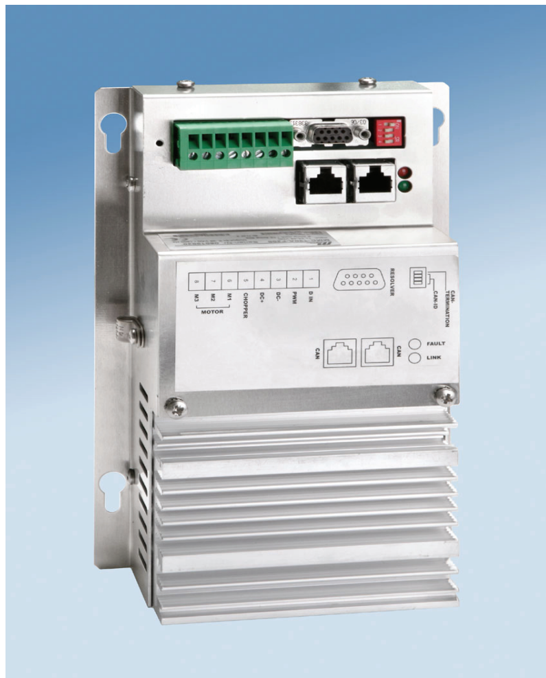
Fig. 7-8 Motor controller MMC-120
